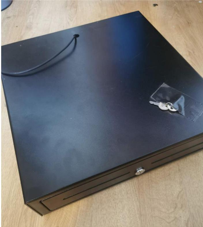
These three pieces of equipment are connected to your computer (PC or laptop) in this order: **Computer -> Customer Display -> Receipt Printer -> Cash drawer**
