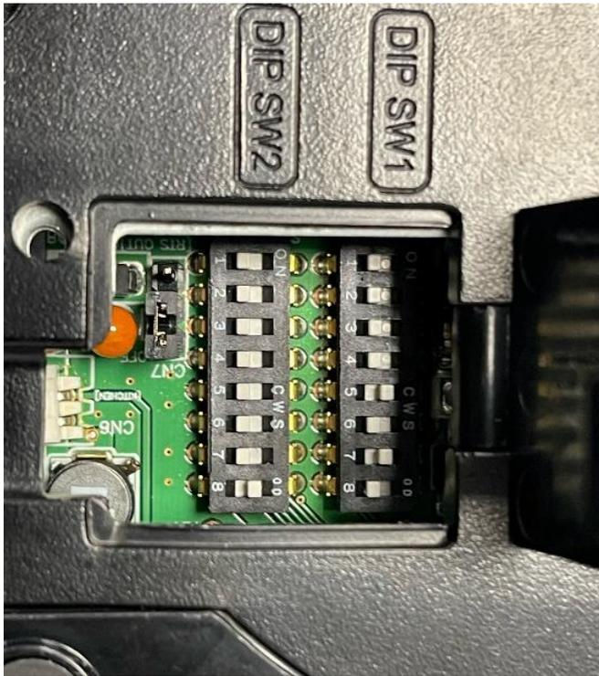
The Dip Switches on the receipt printer (above) should be set as follows:
