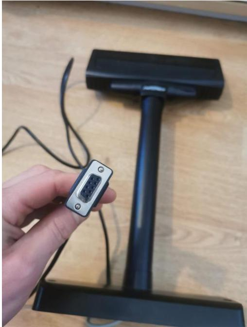
Here is a picture of the customer display being connected to the USB-to-serial port connector:
