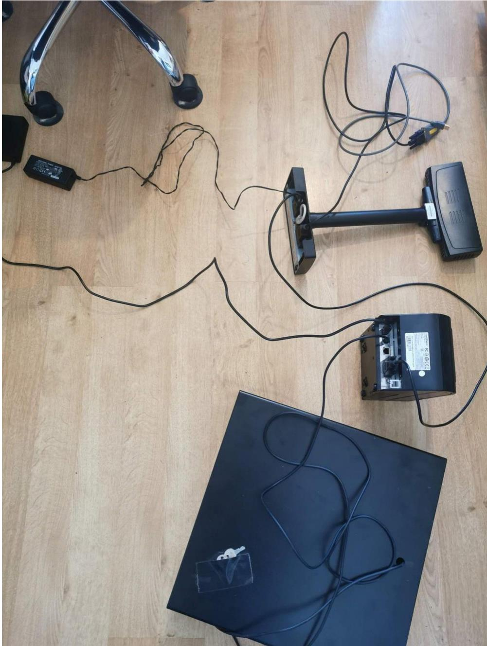
You can also see the two power leads coming from the customer display and receipt printer. These must be connected and powered for the equipment to work properly.
