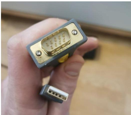
The USB end goes into your computer; the other end will connect to the customer display (or receipt printer if you don't have a customer display).
