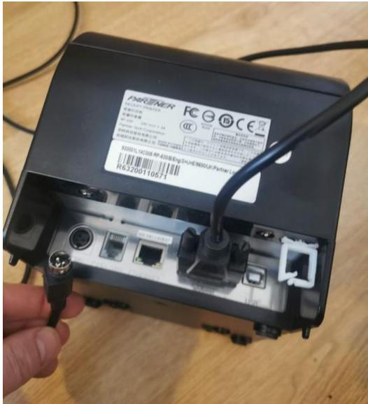
Here is a picture of everything plugged in correctly to the receipt printer. From left to right: Power lead. Cash drawer connector. Connector that goes to the customer display.
