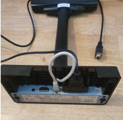
The large connector on the right (above) is the one that connects to the computer, either directly or via a USB-to-serial port adaptor (shown earlier).
